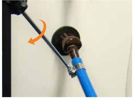
3. Connect the blue air hose to your house air/nitrogen or supply tank. Secure by tightening the metal clamp with a phillips head screwdriver (screwdriver not provided).
