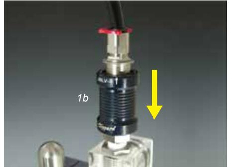
1. To begin, make sure the air flow gauge (1a) is turned all the way off and the main shut-off valve (1b) is in the "off" (down) position.
