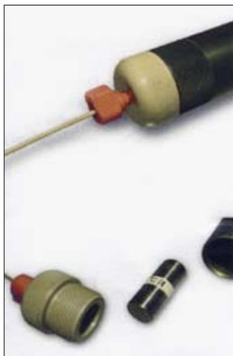
Moisten the free end of the cartridge and reassemble the Holder. Tighten the Holder Ends by hand until they are snug. **Do Not Use Wrenches or Pliers!** The PEEK cartridge end pieces are interchangeable. The knurled end of the aluminum body facilitates opening and closing the Holder and can be used as a flow direction reference after a cartridge is placed in the Holder.
