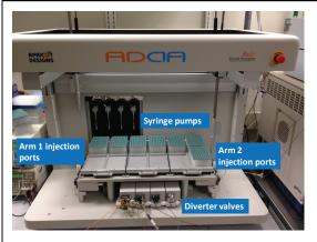
Apricot Designs Dual-Arm autosampler (ADDA) coupled to AB SCIEX API5500 was used for sample analysis.
