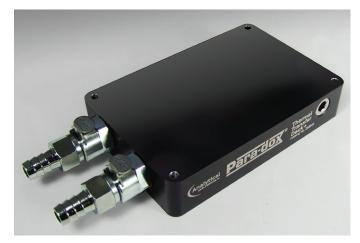
attachment to **solid base** Lumidox® arrays. High-end valved, spill-proof fittings allow for quick connection and disconnection. Input and Output ports are user configurable, and may be relocated between side and top faces. Units are shipped with side exit ports as standard. Decks are stackable, and multiple decks can be chained together for a total temperature control solution.
