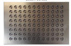
Powder Transfer Plate (cross section view) -Lower plate onto vials and let the vials "settle" into the circular grooves surrounding each hole, essentially locking them in place
