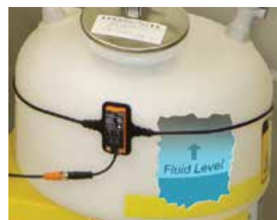
Another sensor can be set to detect high fluid level in your waste container.
