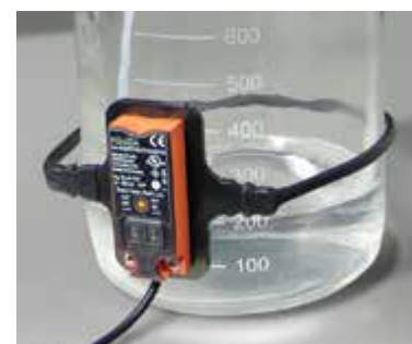
A sensor can be set to detect low fluid level in your mobile phase container.
