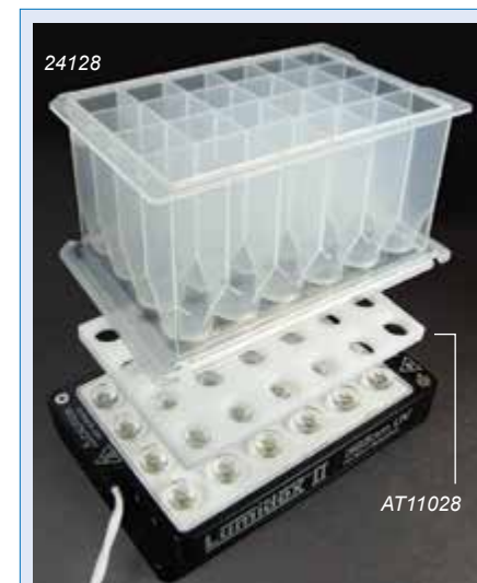
24 well setup with Lumidox 24-well LED Array - See page 72 for array options
