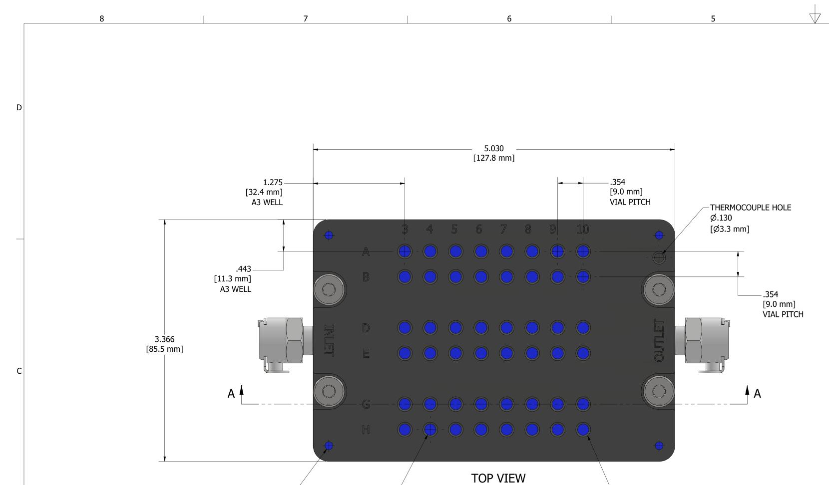
Holes in Lid – LID CORNERS THREADED -Ø.157 6-32 FOR ACCESSORY ATTACHMENT [Ø4.0 mm]
