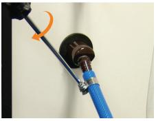
**3.** Connect the blue air hose to your house air/nitrogen or supply tank. Secure by tightening the metal clamp with a phillips head screwdriver (screwdriver not provided).
