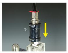
**1.** To begin, make sure the air flow meter *(1a)* is turned all the way off and the main shut-off valve *(1b)* is in the "off" (down) position.
