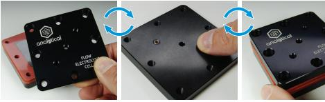
**12.** Find the Lid End Plate. Insert two internal o-rings (F1088301) into the shallow unthreaded diagonal holes (in the side of the plate opposite the logo engraving). Place the Lid End Plate with o-rings on top of the assembled stack, making sure that flow holes are lined up.
