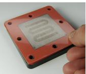
**7.** Add the nafion ion exchange transfer material (F1088201) on top of the flow channel. Ensure that the eight large holes on the sides line up with the those below it.
