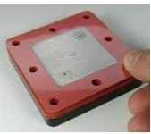
**8.** Place the second isolation layer film on top. **IMPORTANT:** Make sure that the holes in the isolation layer line up with the holes in the Stainless Steel electrode. Do not add a second flow channel.
