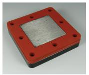
7. Insert the stainless steel electrode (with holes) into the middle space of the silicone gasket. **IMPORTANT:** Make sure that the holes in the electrode line up with the beginning and end of the flow channel.
