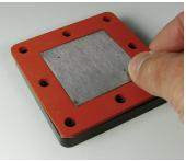
**5.** Insert one electrode into the middle space of the silicone gasket. Make sure that the small diagonal holes in the electrode match the positions of the holes in the base plate and isolation layer.
