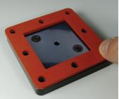
**3.** Place one silicone gasket (F1088504) on top of the Base Plate and Isolation Layer Film.
