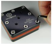
**13.** Insert 8 M6 screws through the holes of the lid plate and those of the layers beneath it, then screw them into the bottom plate with an alan wrench.
