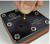
2. With the flow electrolysis cell fully assembled, gently place the pogo pin / ferrule assembly into the center hole of the end plate. Ensure that the spiked head of the pogo has is making contact with the electrode.
