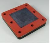
**10.** Insert the second electrode, making sure that the holes line up with the beginning and end of the second flow channel (alignment with flow holes of previous layers not necessary).
