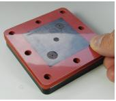
**11.** Add the second isolation layer, making sure that the holes line up with the holes of the second electrode.
