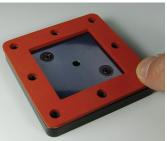
**4.** Place one silicone gasket (F1088504) on top of the Base Plate and Isolation Layer Film.
