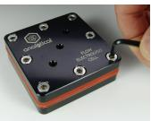
**10.** Insert 8 M6 screws through the holes of the lid plate and the layers beneath it, then screw them into the bottom plate with an alan wrench.
