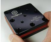
**9.** Find the Lid Plate. Insert two internal o-rings (F1088301) into the shallow unthreaded diagonal holes (in the side of the plate opposite the logo engraving). Place the Lid Plate with o-rings on top of the assembled stack, making sure that flow holes are lined up. **Tip:** use your thumb or finger to press the o-rings into the holes. This will help keep them in place when placing the lid plate onto the assembly.
