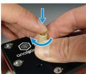
**3.** Slide a fitting around the pogo pin. With the fitting held free, press the top of the pogo pin down so that it bottoms out on the electrode and then begin twisting the fitting. Continue to press on the top of the pogo pin until the fitting is tight on the ferrule.
