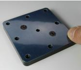
**2.** Place one 0.010" PFA Isolation Layer Film (F1088405) on top of the base plate. Make sure that all holes on the Isolation Layer are aligned with those of the base plate.
