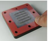
**8.** Place the second flow channel film (from set of 2) on top of the ion exchange film.
