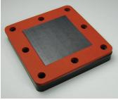
**4.** Insert the graphite electrode (with no holes) into the middle space of the silicone gasket.
