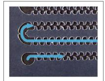
**Note:** If using F1088410, ensure that the flow channel is oriented so that the fins are pointing into the path of the fluid (see diagram).
