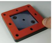
**4.** Place one silicone gasket (F1088504) on top of the Base Plate and Isolation Layer Film.
