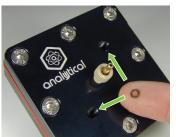
**5.** Insert the external o-rings (F1088302) into the deep diagonally positioned holes in the Lid and Base End Plates. These are where the fluid connections will be made.
