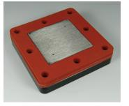
7. Insert the stainless steel electrode (with holes) into the middle space of the silicone gasket. **IMPORTANT:** Make sure that the holes in the electrode line up with the beginning and end of the flow channel.
