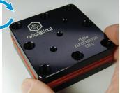
**12.** Find the Lid End Plate. Insert two internal o-rings (F1088301) into the shallow unthreaded diagonal holes (in the side of the plate opposite the logo engraving). Place the Lid End Plate with o-rings on top of the assembled stack, making sure that flow holes are lined up.
