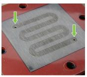
**6.** Choose a Flow Channel Film set from the 4 sets provided (F1088407, F1088403, F1088410, or F1088406). Place one flow channel film on top of the silicone gasket/electrode. **IMPORTANT:** Make sure that the beginning and end of the flow channel line up with the flow holes in the base plate/isolation layer/electrode.
