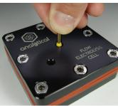
**2.** With the flow electrolysis cell fully assembled, gently place the pogo pin / ferrule assembly into the center hole of the end plate. Ensure that the spiked head of the pogo has is making contact with the electrode.
