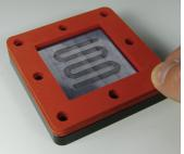
**6.** Place the second silicone gasket on top of the flow channel film.
