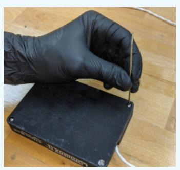
**STEP 1:** Turn the Lumidox II LED array over, and using a 1/16" Allen key, remove the 4 screws securing the bottom plate.
