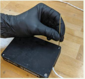
**STEP 2:** Using the same 1/16" Allen key, secure the bottom plate of the Lumidox II with the 4 shorter screws.
