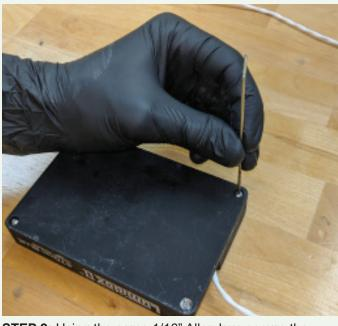
**STEP 2:** Using the same 1/16" Allen key, secure the bottom plate of the Lumidox II with the 4 shorter screws\* originally provided with your array.
