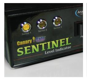
Front panel LEDs indicate which sensor has been activated.
