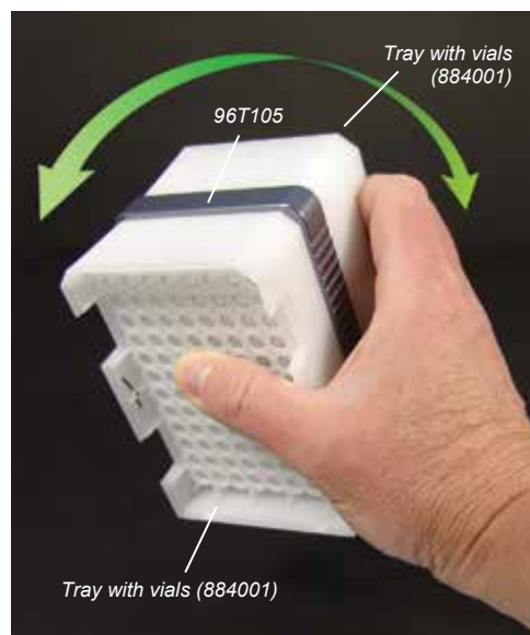
Flip repeatedly to mix powders between vials
